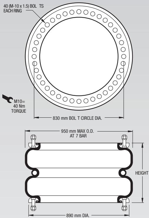
**NOTE:** The effective length of the 45 mm bolt is 30 mm in this bead ring.
